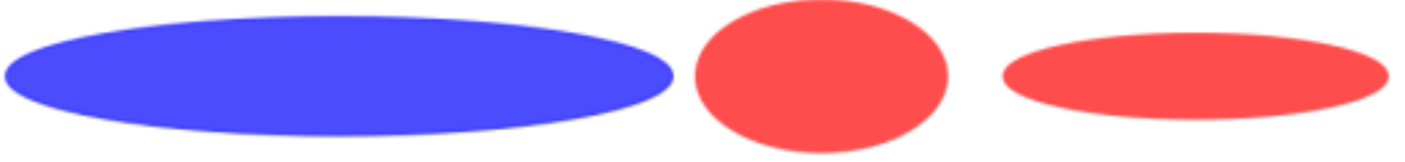
FIG. 42. Apparent horizontal broadening of the beam spot size at the IP due to the crab tilt. Blue left: RMS hadron bunch length \sim 10\text{cm} , red middle: Looking along the beam with no crabbing, and red right: What the RP sees \sim 1.25\text{mm} .
